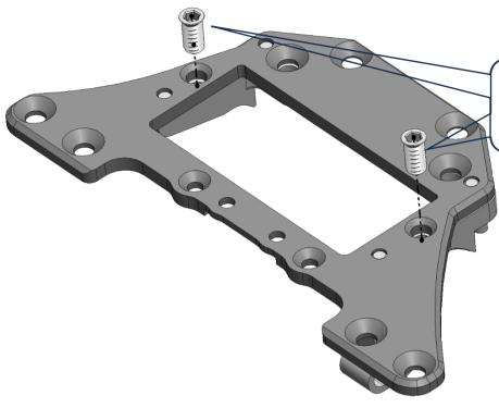
The provided Small Head Countersunk screw is used at this position to fix the motor mount.
