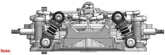
To have a good performance and stable car, the key point is to make sure there is "No droop" no matter what ride height the front it is. That means, the front arm is not able to drop down if you lift the car. Adjust it thru the "droop screw" of the lower arm to achieve this. (If you sway Bar is installed, the situation is different. it needs some droop to work well)
